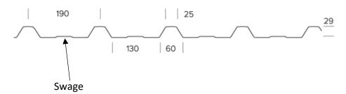
[17] The effective difference between the two products is that the T-Rib product only has one swage, and the installed product has a 2mm deeper trough. A swage is a raised rib used to minimise distortion.
